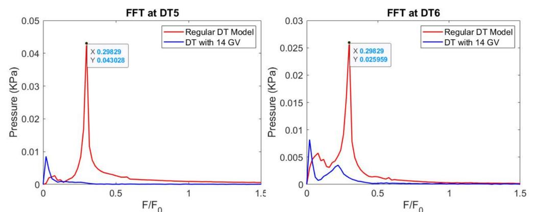
Figure 4: Comparative FFT results between the reference DT model and the draft tube with GVs.
