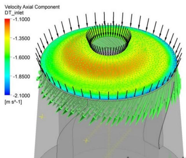
Figure 2: Reduced Draft tube model of Francis-99 turbine.
