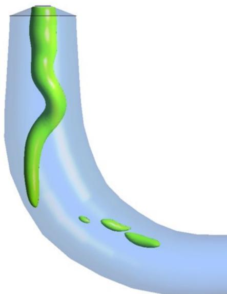
Figure 1: Rotating Vortex Rope (RVR) inside Draft tube
