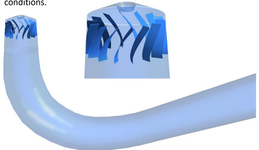
Figure 3: Preliminary design of the draft tube with GV.
